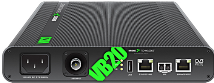
Figure - The VB20 portable IP Probe with ASI input, 10/100/1000-T RJ45 management, 10/100/1000-T RJ45 video and SFP video port. 100-240VAC PSU is built-in. Unit is fanless and dissipates approximately 15W of power.
